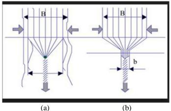
Figure 3. Spinning triangle of (a) Ring spinning (b) Compact spinning
