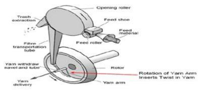
Figure 4. Principle of Rotor spinning
