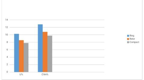
Figure 5. Comparison of mass variation among ring, rotor and compact yarn (From Table 2)
