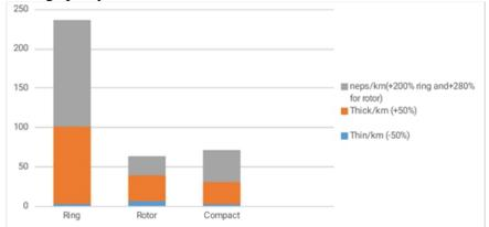
Figure 6. Comparison of imperfection among ring rotor and compact yarn (From Table 2)
