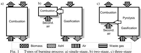
Types of burning process: a) single-stage, b) two-stage, c) three-stage
