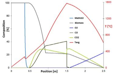
Fig. 8 Results of the simulations for alternative 2 – production of "Syngas"
