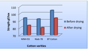
Fig 3.9 Effect of storage on Bundle strength of cotton fibers
