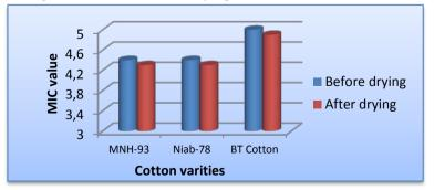
Fig 3.5 Effect of artificial drying on fineness of cotton fibers
