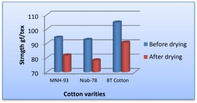
Fig 3.8 Effect of artificial drying on Bundle strength of cotton fibers
