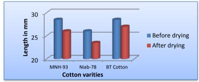
Fig 3.2 Effect of artificial drying on Effective Length of cotton fibers
