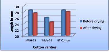
Fig 3.1 Effect of natural drying on Effective Length of cotton fibers
