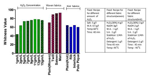
Figure-4: Whiteness of cotton fabrics for different concentration of  $H_2O_2$  & fabric structures
